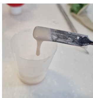
FIGURE 6: Checking the flow and consistency of the mix.
